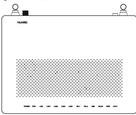
Figure 1-6 LEDs on the HG8247H
